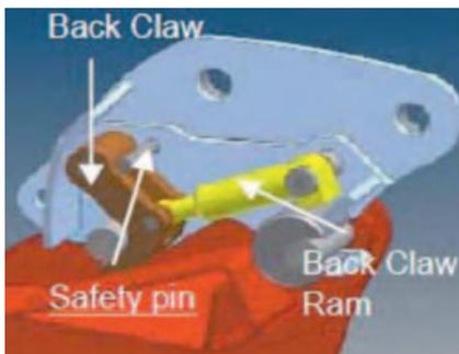
Figure 3 – Semi-automatic quick hitch
