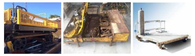
Similar risks (although lower potential) may also apply to other light weight rail trolleys such as machine support frames and hand held measuring trolleys. If left unattended these items should have tooling grounded or be totally removed from the running line.
