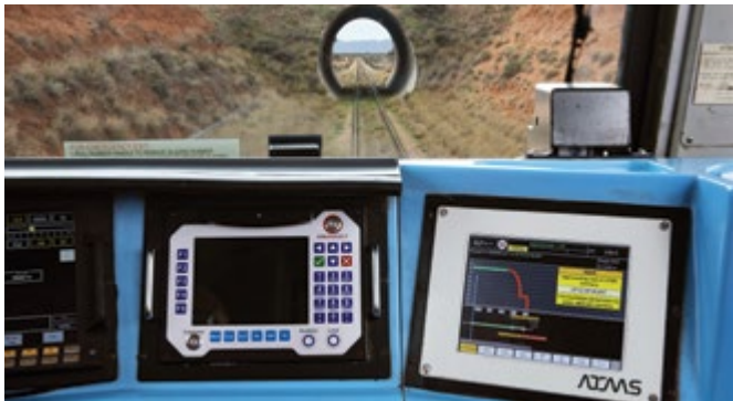
Figure 5: Driver Management Computer/Display
