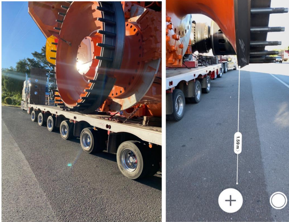
Oversized load (mining haul truck on heavy haulage float) and the vehicle impact point.
