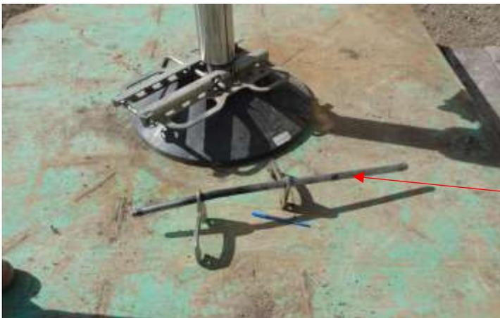
Photo indicates the guide bar that fell 10m and the position where it landed.
