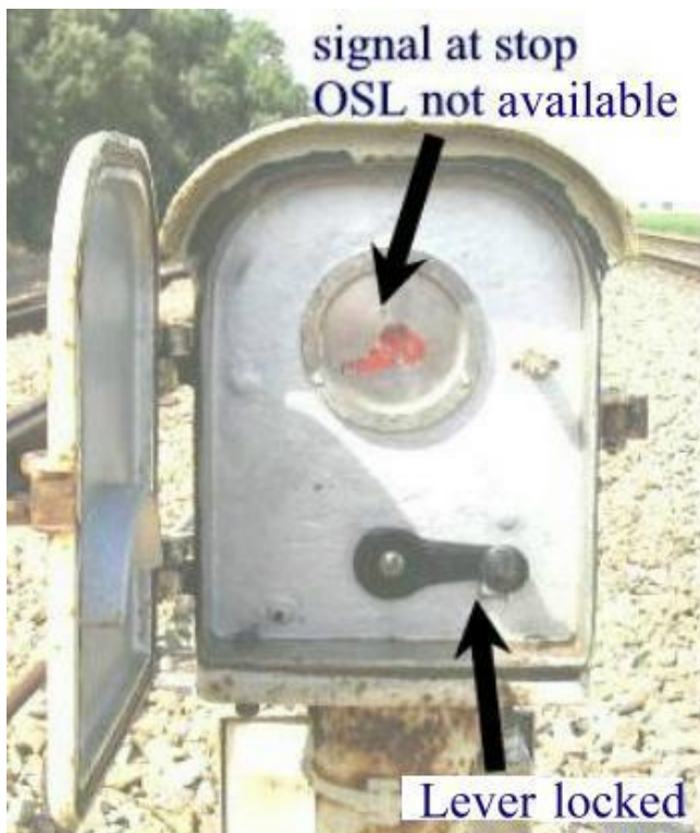
OSL with indicator at stop and lever locked.
