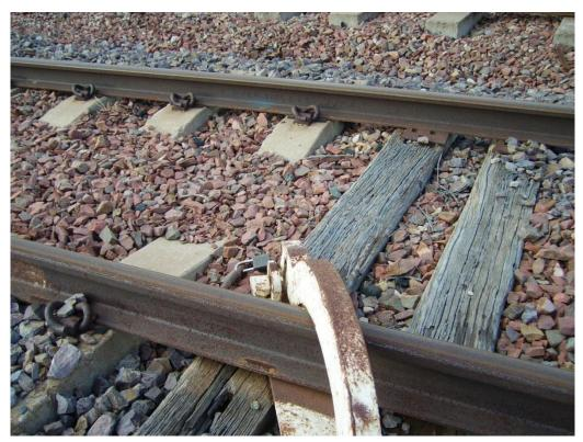
Derailers are placed on goods sidings for roll out protection.
