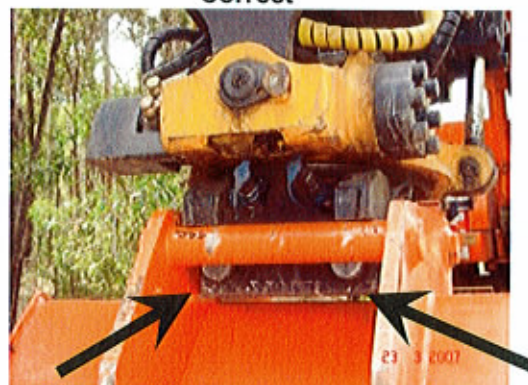
Photo 2 Bucket Correct Installed
