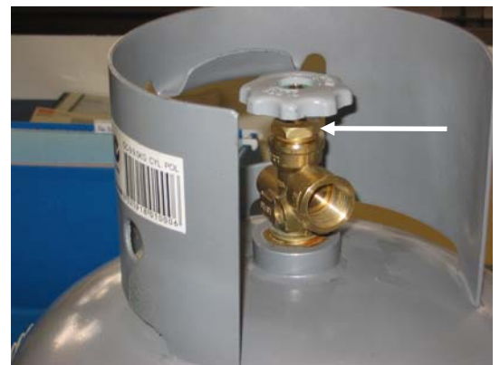
Valve showing loose gland nut
