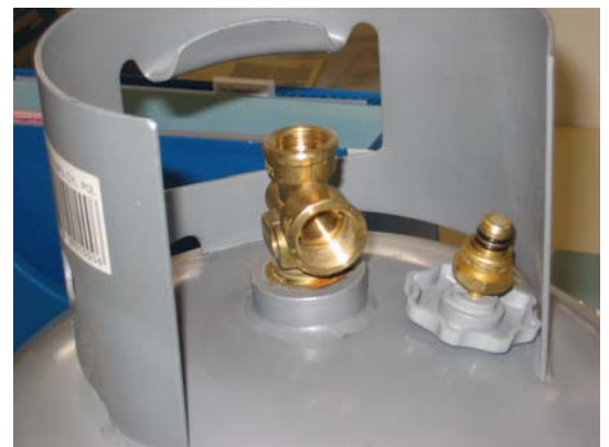
Valve can fall apart during closing action
