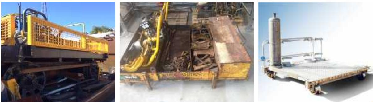
Similar risks (although lower potential) may also apply to other light weight rail trolleys such as machine support frames and hand held measuring trolleys. If left unattended these items should have tooling grounded or be totally removed from the running line.
