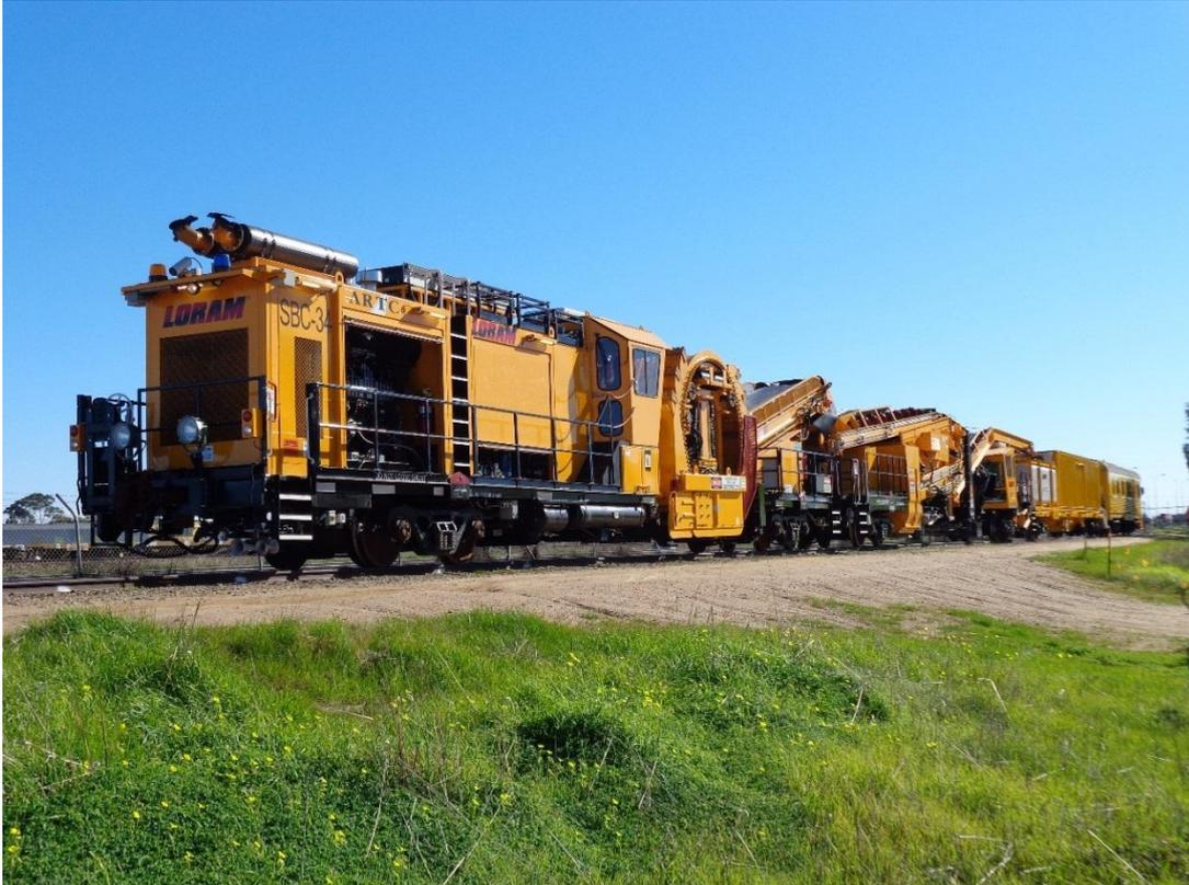
The Loram HP Shoulder Ballast Cleaner is a self-powered heavy duty machine that uses twin 660mm-wide digging buckets to clean ballast from the sleeper ends outward to the edge of the ballast section, digging as deep as 400mm below the top of sleeper. Scarifier teeth undercut the sleeper ends to 125mm, breaking up mud pockets and restoring drainage.
